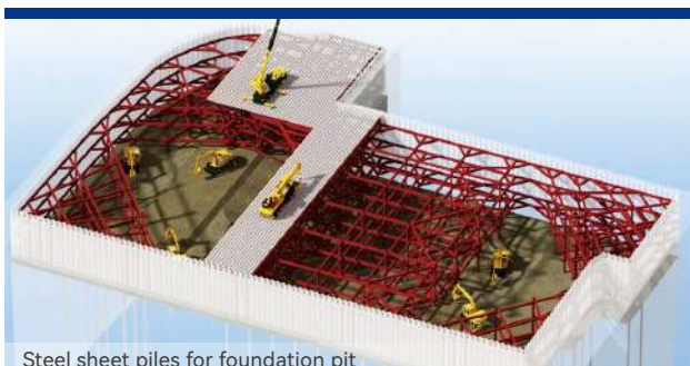
Steel sheet piles for foundation pit
